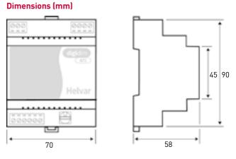
DIN rail housing; The width of 4 modules. Weight 140 g
