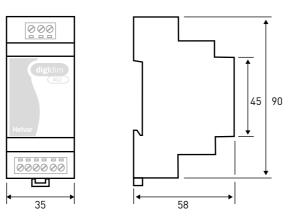
DIN rail housing; Width of 2 modules. Weight 80 g
