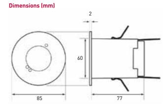
The diameter of the mounting hole: 75 mm White plastic, weight 100g
