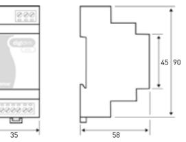
DIN rail housing; Width of 2 modules. Weight 110 g
