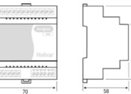
DIN rail housing; The width of 4 modules, Weight 110g
