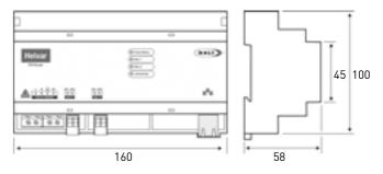
DIN rail housing; Width of 9 modules. Weight 260 g
