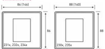
() = dimensions of the double frame Frame weight: 100 g (144 g) Panel weight: 41 g
